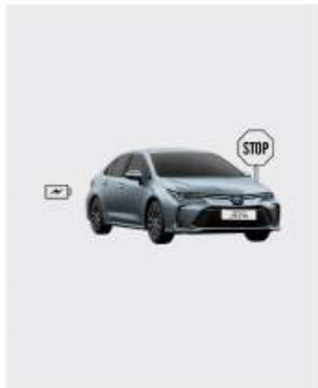
IDLE/LOW SPEEDS When sufficiently charged, the battery powers the vehicle to save fuel.
